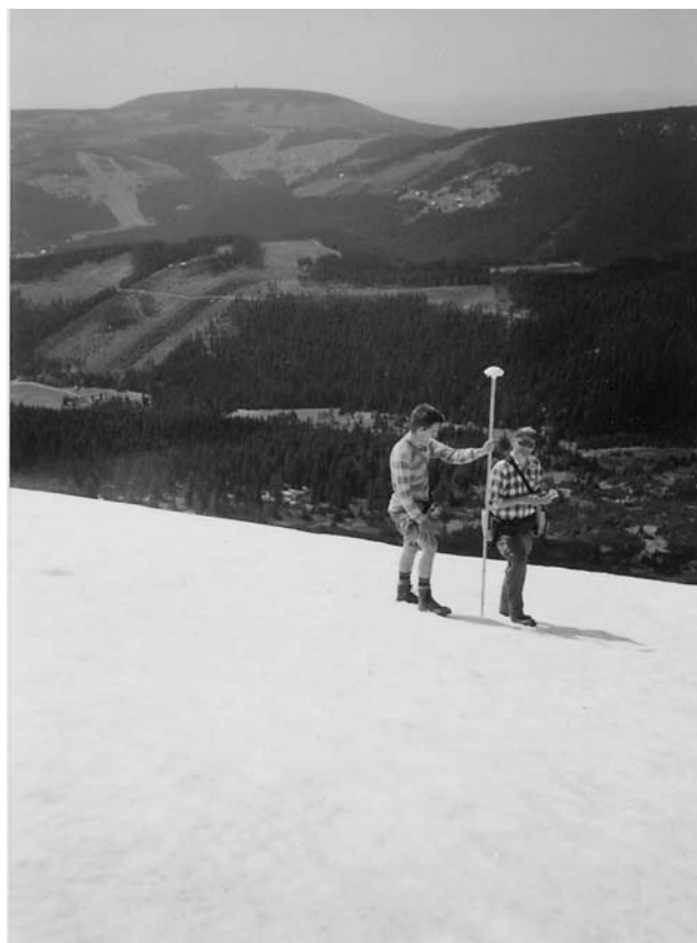
FIGURE 2. Kinematic GPS measurement by “stop and go” method on the investigated snowbed in May 2000; each point was recorded in the course of 30 sec; antenna height of the GPS receiver was 2 m.
